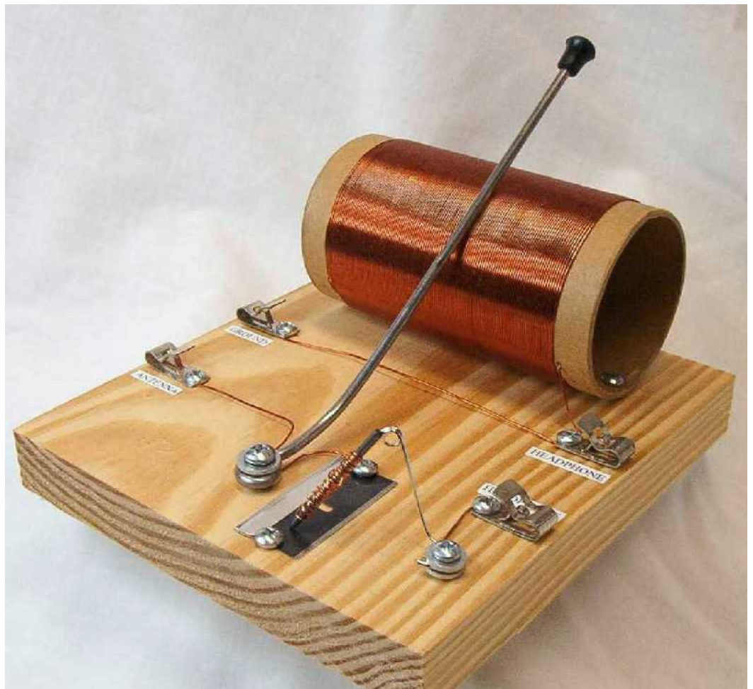
Homemade foxhole radio from modern components
